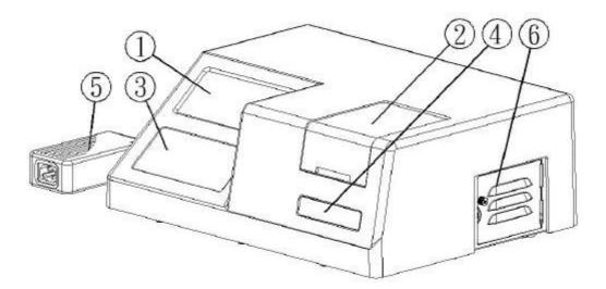
Figure 1: Components of SP880 spectrophotometer
