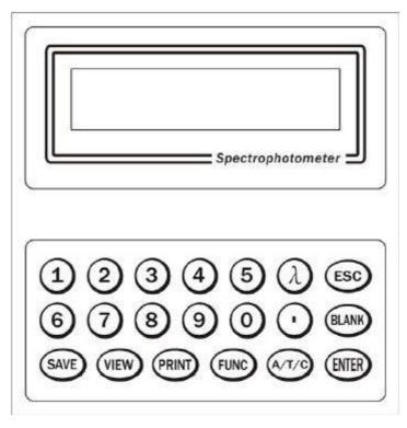
Figure 2: Keyboard and display layout
