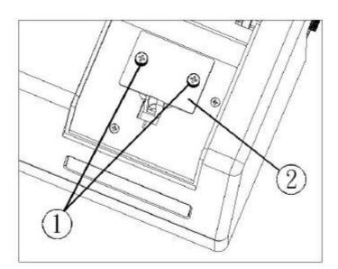
Figure 4a: Standard cell holder for  $10 \sim 13$  mm cuvettes
