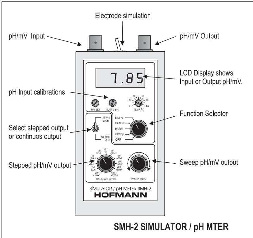
The OFFSET, SLOPE and TEMP. adjustments let you calibrate an electrode to achieve accurate measurements on site.
