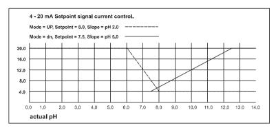
FIG 10 4-20mA Setpoint Signal current control.
