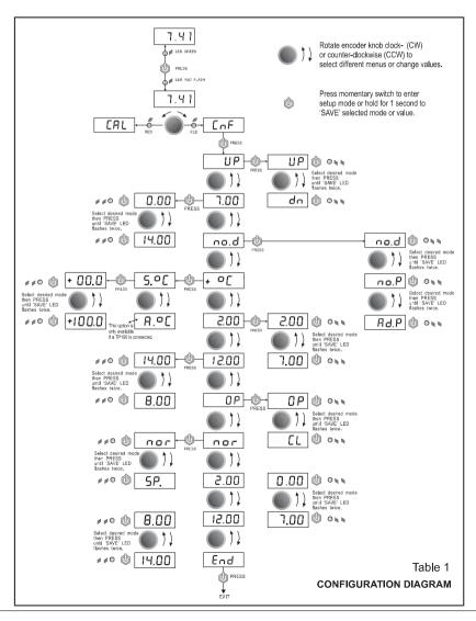
When dialing up numbers such as the setpoint, the encoder steps in single digits if turned slowly. To change large numbers quickly rotate the encoder in a "flicking" manner.
