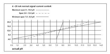
FIG 9 4-20mA normal Signal current control.
