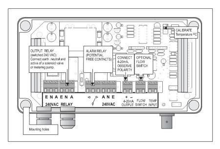
FIG 5 Terminal layout of the PPH-1.
