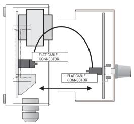
FIG 3 CHASSIS & removable FACIA of the PPH-1
