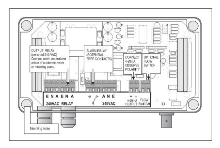
FIG 5 Terminal layout of the PMV-1.
