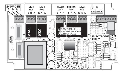
The Set point relay terminals connect to earth, neutral and switched active 240V. (240VAC is supplied to these terminals when activated by the set point.)
