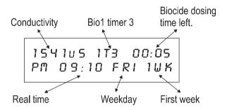
The timers are identified in the display window during a biocide cycle. The remaining biodosing time is displayed on the top line, right side. Which timer calls the biodosing is indicated as 1T1, 1T2, 1T3, 1T4, 1T5 or 1T6.
