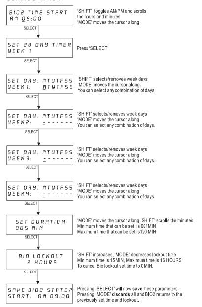
This feature greatly helps the efficiency of operation as you only scroll through the active timer configurations.
